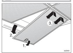
■ To remove the grease filter pull the locking clips forward 1., lower the filter down 45° 2., unhook it at the rear 3., and take it out.
