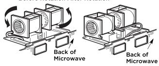
5 Gently remove the wires from the grooves. Reroute the wires through grooves on other side of the blower unit.
