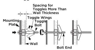
and insert the toggle wings into the holes in the wall to mount the plate.
