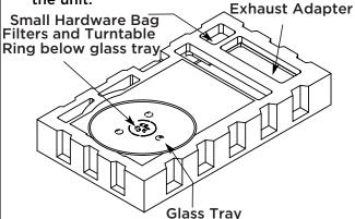
2 Fold back all 4 carton flaps fully against carton sides. Then carefully roll the oven and carton over onto the top side. The oven should be resting in the Styrofoam.
