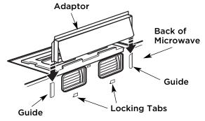
Push in securely until it is in the lower locking tabs. Take care to assure that the damper hinge is installed so that it is at the top and that the damper swings freely.
