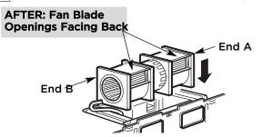
CAUTION: Do not pull or stretch the blower unit wiring. Make sure the wires are not pinched, and that they are properly secured.
