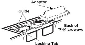
Push in securely until it is in the locking tabs. Take care to assure that the damper hinge is installed so that the damper swings freely.
