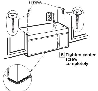
7 Tighten the outer two screws to the top of the microwave oven. (While tightening screws, hold the microwave oven in place against the wall and the top cabinet.)
