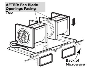
CAUTION: Do not pull or stretch the blower unit wiring. Make sure the wires are not pinched, and that they are properly secured.
