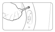
Re-attach the remaining screws to the remaining holes above and below the lever holder, and then tighten.
