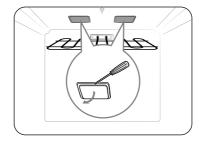
While holding the glass cover with one hand, insert a flat-sharp tool such as a table knife between the glass and the frame to remove the glass cover.
