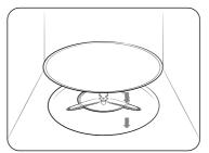
Remove all packing materials inside the oven. Install the roller ring and turntable. Check that the turntable rotates freely.
