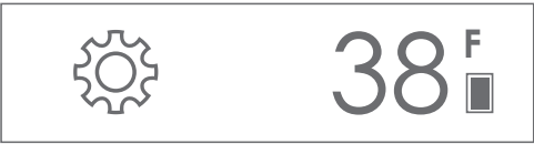
Single-zone refrigeration display
