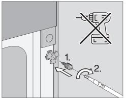
■ Insert the bolt into the mounting aid and tighten it in the cabinet niche. **Do not** use a cordless screwdriver.
