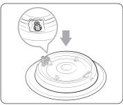
2. Install the burner head so that the electrode passes through the opening for the electrode. Make sure the burner head lies flat on the stove top.
