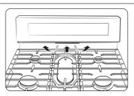
The oven vent is located under the oven Control panel. Proper air circulation prevents oven burner combustion problems and ensures good performance.
