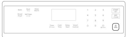
Press and hold the 🔁 for 3 seconds to lock or unlock both the control panel and the door. When the Oven Lock is on, the oven panel does not operate and the oven door is locked and cannot be opened.
