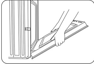
4. Lower the oven door to the fully open position. If the oven door does not open to a full 90°, repeat steps 1 through 3.
