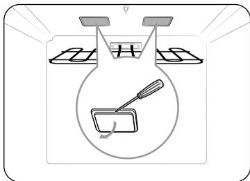
2. While holding the glass cover with one hand, insert a flat-sharp tool such as a table knife between the glass and the frame to remove the glass cover.
