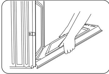
4. Partially close the door to engage the door latch locks. The door will stop at this point.
