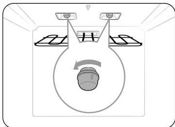
3. Turn the bulb cap counterclockwise to remove.
