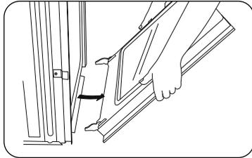
5. Using two hands, grasp the edges of the oven door. Lift and pull the oven door toward you and remove. You may need to gently shift the door from side to side as you pull.
