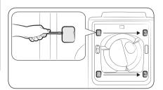
**6.** Use a flat-head screwdriver to remove the two hinge covers from the original side. Install the hinge covers on the opposite side as shown.
