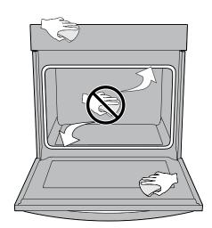
Figure 14: Clean around the oven door gasket
