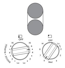
4. Push in and turn the Bridge ON/OFF knob to ON position to switch on bridge element.
