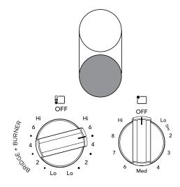
3. Push in and turn the left rear element control knob to the desired setting.
