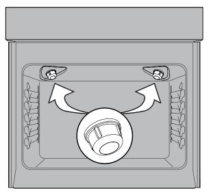
Figure 19: Oven Halogen light
