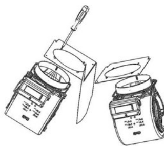
Figure C: Connect Blowers Install dual 600 CFM blowers onto mounting plates with included hardware.
