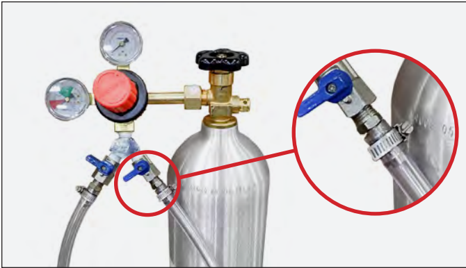
FIG. 7. Installed pressure regulator and air hoses. Be sure the hose clamps are tightened to prevent leaks.
