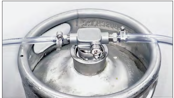
FIG. 10. Installed and connected tapper. Be sure the hose clamps are tightened to prevent links.
