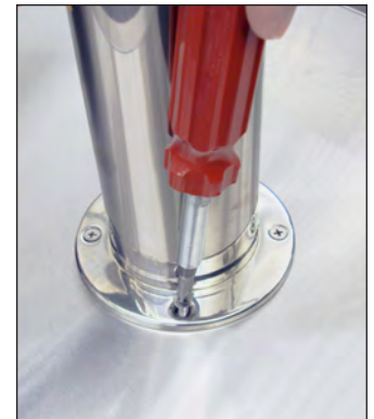
FIG. 3. Secure the draft standard to the countertop.
