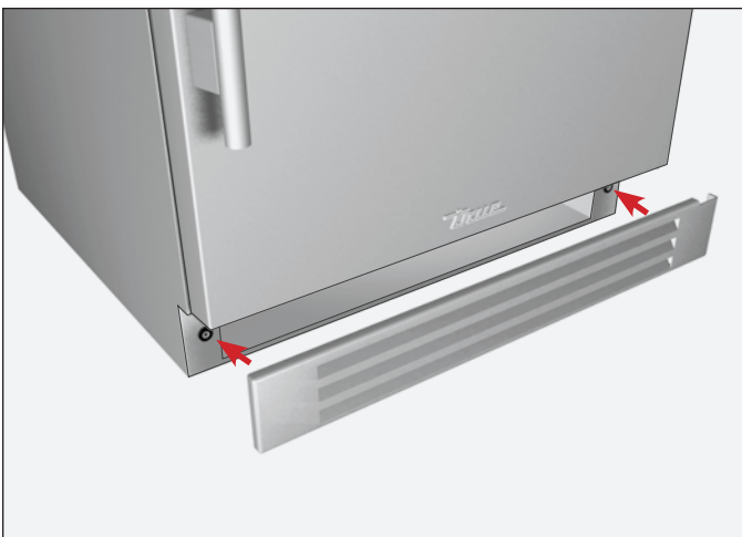
FIG. 2. Attach the kickplate to the magnets below the door.
