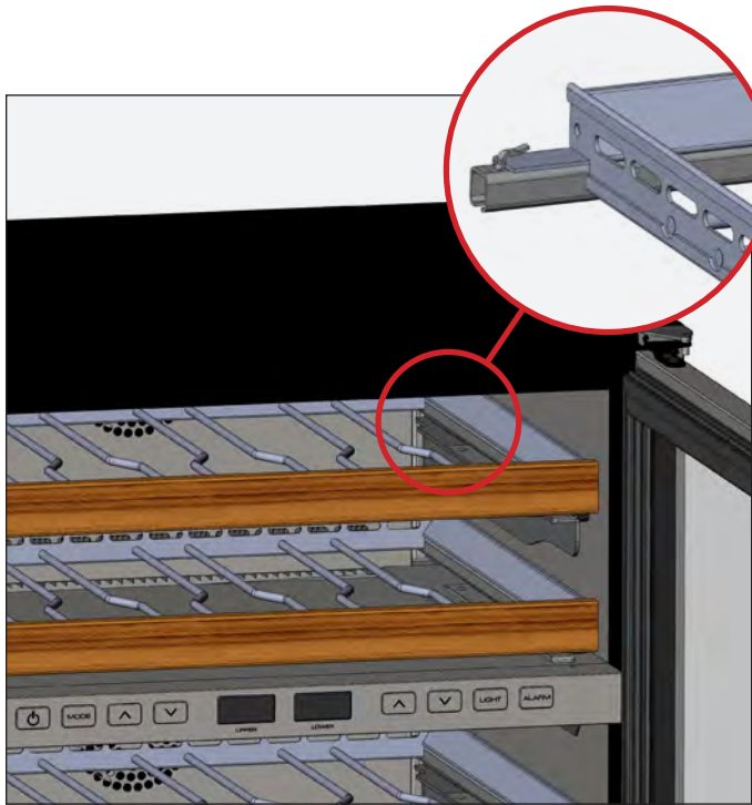
FIG. 4. Be sure the wine rack sits under the rear tabs.
