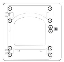
7. Locate and remove the 10 screws as shown. Note that screw B (x2) is longer than the others.
